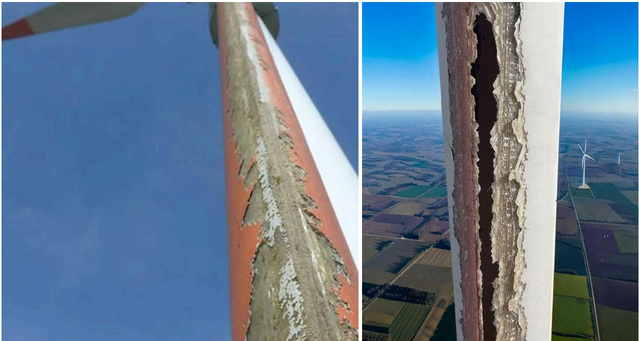
Leading edge erosion from bad to worse
