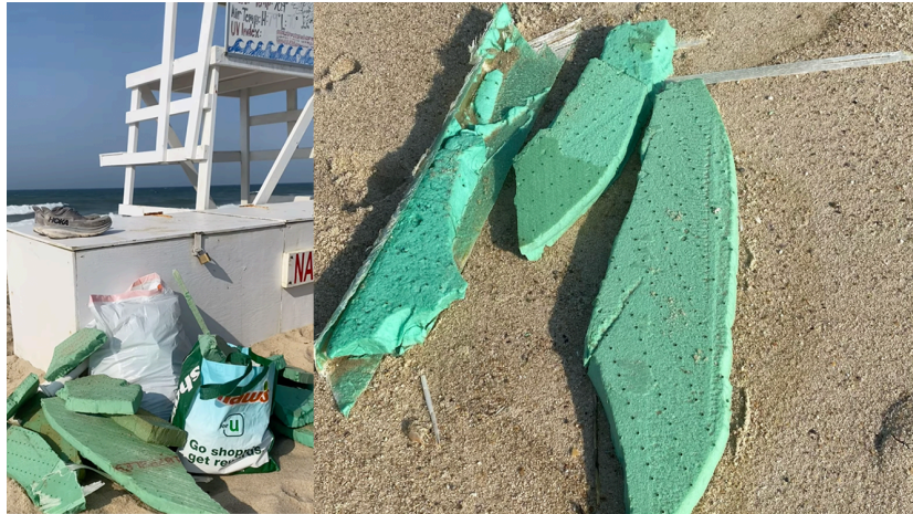
PET Foam in Nantucket blade failure debris
